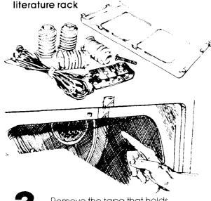
Remove the tape that holds the drum to the cabinet. (Some dryer drums are not taped for shipping.) Move the drum by hand to make certain all tape has been removed. Wipe the interior of the drum thoroughly with a damp cloth before using the dryer.
